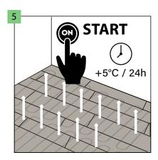
After laying the floor and waiting 24 hours, you can turn on the underfloor heating, remembering to gradually increase the temperature (5°C per day).
