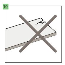
Before and during the installation, control all the panels in the optimal lighting conditions. Do not use defective panels.
