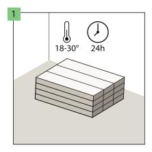
It is recommended to maintain caution during the transport and storage of panels. It is recommended to transport and store the product in a lying position. The packaging must not be placed vertically, stored in wet or dusty premises or in locations exposed to the impact of extreme temperatures.
